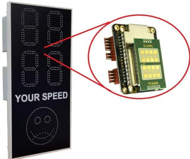
CW Doppler device operating in the K-Band (24GHz)
