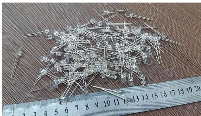
LED's are identified very well and amount of their desired life is 100.000 hours in lawful range for traffic light and traffic signals and its light intensity is 8000mcd. Total numbers of LEDs in one device are equal to 507pcs for Seven Segment and Emoji face plus LED for messages.
