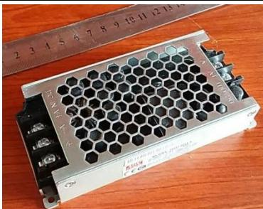
We used DC to DC converter for preparing of 5 volt from 12 volt to supplying LED display modules. This is manufactured by Meanwell company.
