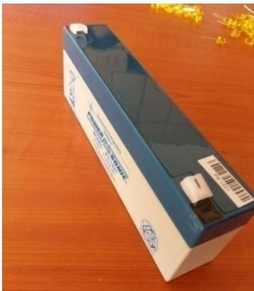
Sealed Lead Acid batteries of 2x12v \*18Ah, totally 36Ah, having desired life of 5 years.
