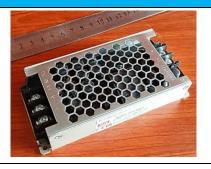
We used DC to DC converter for preparing of 5 volt from 12 volt to supplying LED display modules. This is manufactured by Mean well company.
