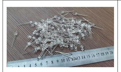
LED's are identified very well and amount of their desired life is 100.000 hours in lawful range for traffic light and traffic signals and its light intensity is 8000mcd.
